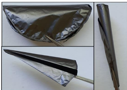
Figure 1. Illustrative digital photo of the flexible and shapeable \text{NiCo}_2\text{S}_4/\text{rGOP} .
