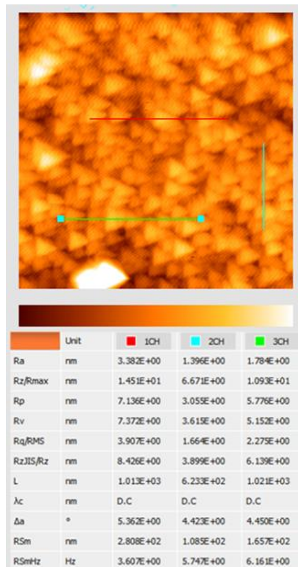
Fig. 5. AFM image of 300 °C 100 mTorr sample
