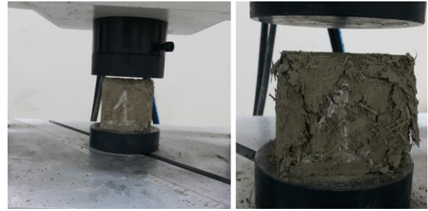
Fig. 9. Compressive strength test of adobe block
