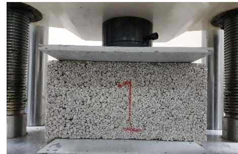
Fig. 5. Compressive strength test on bims block
