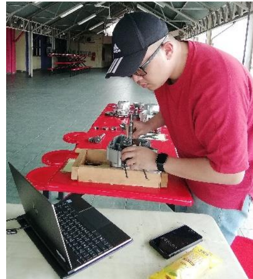
Fig. 1. Video-guideline based automobile engine assembly.
