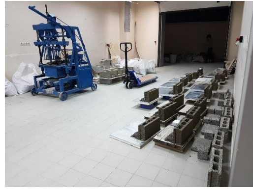
Fig.7. Single bims block productions at the laboratory
