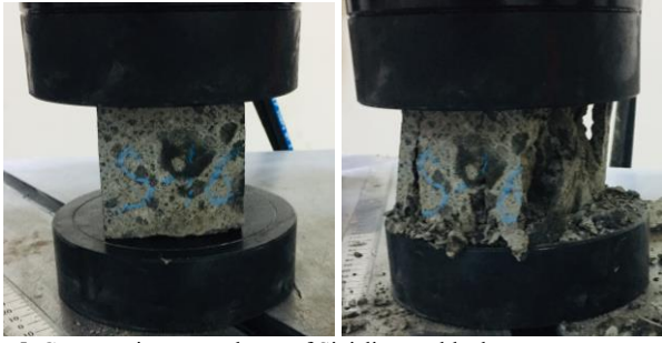
Fig. 5. Compressive strength test of Sivişli stone block
