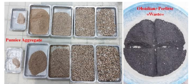
Fig. 6. Aggregate used for lightweight concrete production
