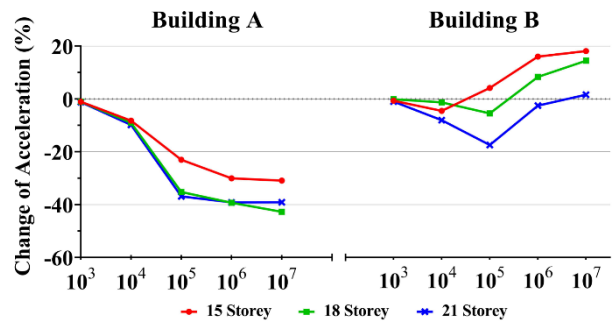
Fig. 8. The change of the acceleration of the top floor (Soil Type I).
