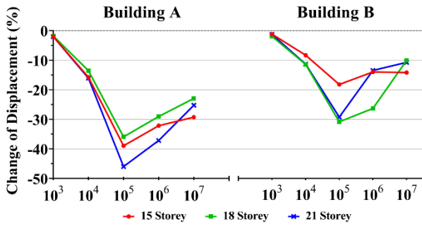
Fig. 9. The change of the displacement of the top floor (Soil Type II).
