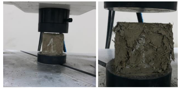
Fig. 9. Compressive strength test of adobe block
