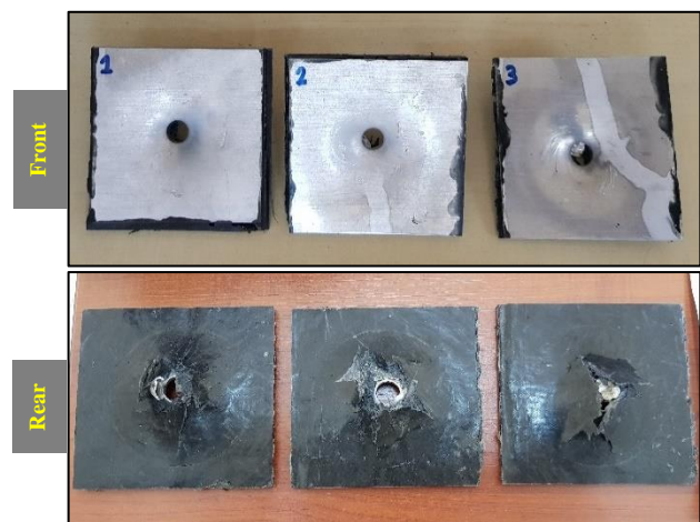
Fig. 9. Perforation damage of the bilayer plate with hemispherical punch
