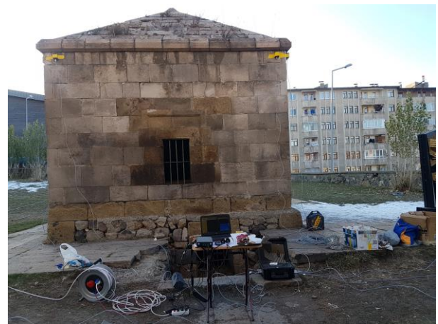
Fig. 8. Instrumentation for acceleration response measurement of the historic cupola
