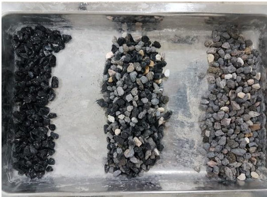
Fig.9. Obsidian and gabbro particles existing in pumice aggregate
