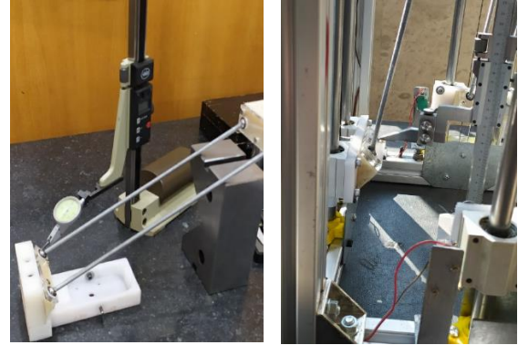
Fig. 5. Measurement and calibration process of manipulator under study.
