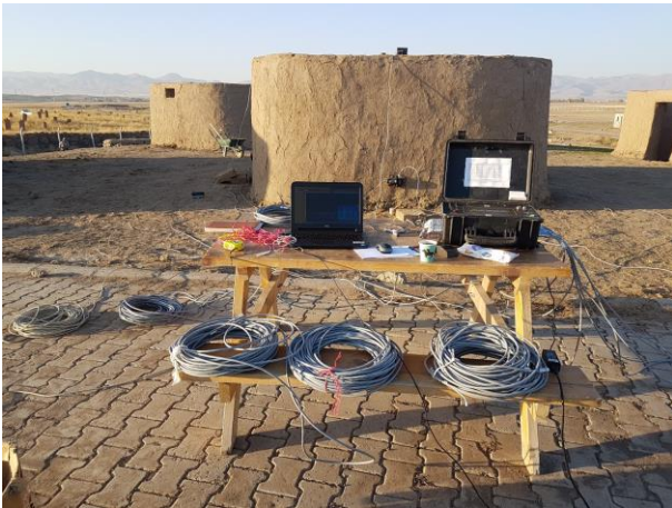
Fig. 11. Instrumentation for acceleration response measurement of adobe cottage
