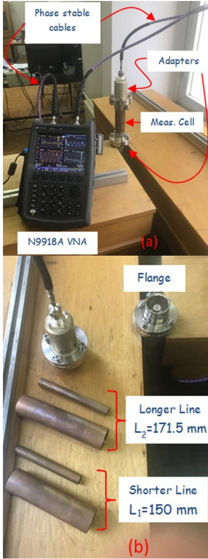
Fig. 2. (a) A picture of the measurement setup and (b) a picture of the shorter and longer coaxial lines with L_1 = 150 mm and L_2 = 171.5 mm.
