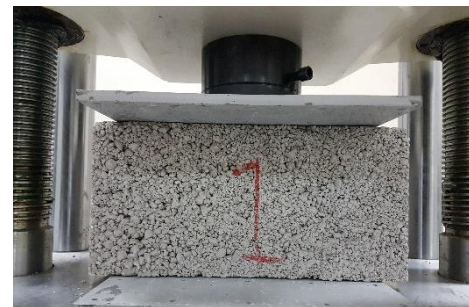
Fig. 5. Compressive strength test on bims block
