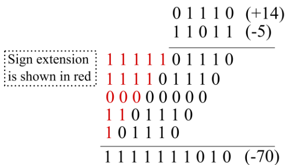
Fig. 3. Signed combinational multiplier with sign extension.
