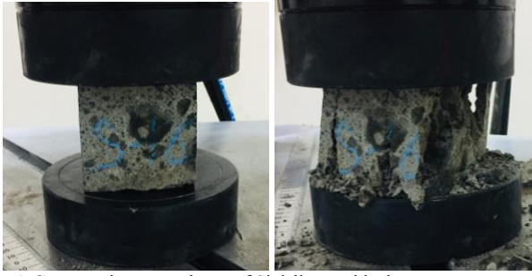
Fig. 5. Compressive strength test of Sivişli stone block
