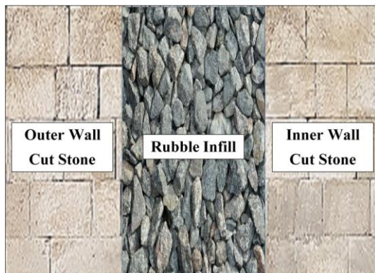
Fig.7. Schematic view of cupola wall section
