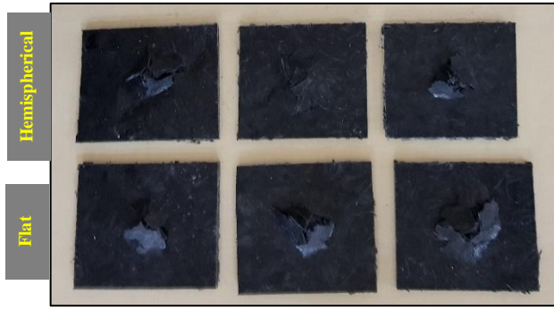
Fig. 6. Perforation damage of the rear faces for the composite samples
