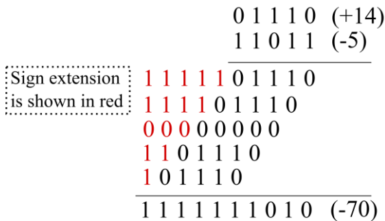
Fig. 3. Signed combinational multiplier with sign extension.
