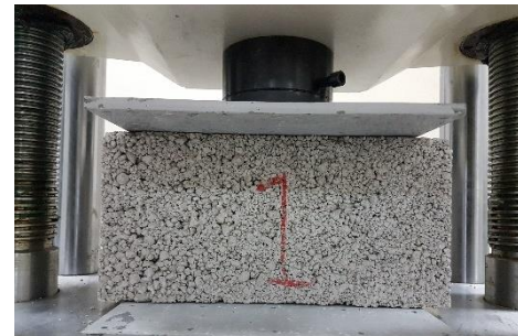
Fig. 5. Compressive strength test on bims block
