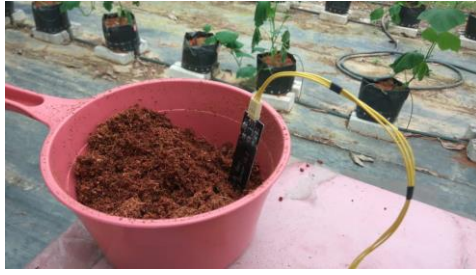
Fig. 4. The moisture sensor is placed in a bucket of fertilizers.
