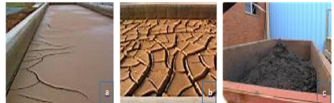
Fig. 1. Figures below are from different sludge dewatering methods. a) Sludge drying bed, b) Vakum filtration, c) Sludge belt press
