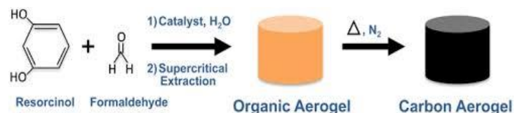
Fig. 2. Carbon Aerogel Synthesis Procedure
